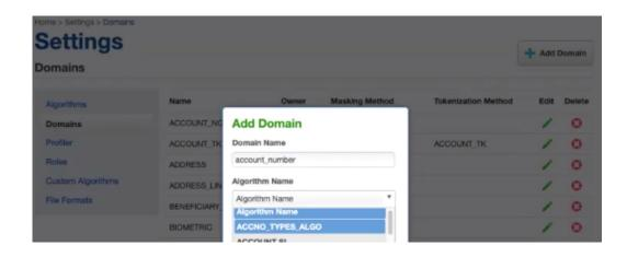
4) Assign masking algorithms to the columns to be masked
